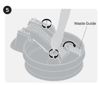
5. Lower the conveyor and tighten the thumb screws, then flip the waste guide down into place.
