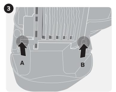
Install the conveyor by sliding the long post at the top (A) into the hole on the conveyor base. Then insert the short post (B) on the opposite side into the hole in the base by pressing it down into the hole with the flange pointing down.
