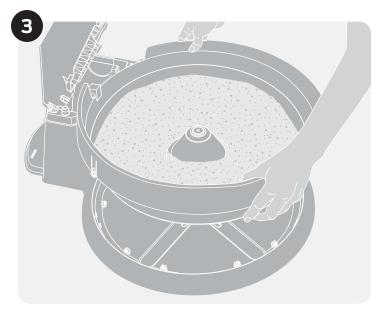
3. Lift up the litter bowl to remove it, and dispose of the used litter.
