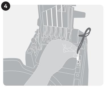
4. Leave the conveyor in the upright position, and plug in the motor. The motor plug is at the end of the red wire, and it clips into the conveyor base.
