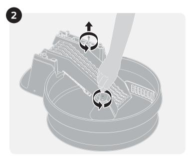
2. Remove the thumb screws from the center of the litter bowl and top of the conveyor. Lift the conveyor to its upright position.
