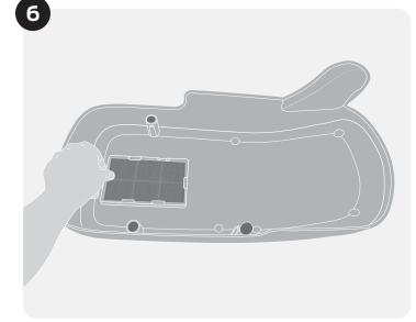
6. Place one carbon filter into the brackets on the inside of the conveyor cover. The black side of the filter should face outward. The carbon filter helps reduce odors from the waste trap area. Place the conveyor cover over the conveyor, making sure it is secure.
