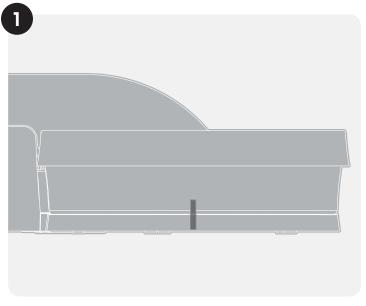
1. To test if the litter box is rotating properly, place one piece of adhesive tape on the base of the unit and one piece of tape on the bowl of the unit.
