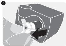
7. Rinse the carbon filter and insert it into the housing with the black side facing the pump.
