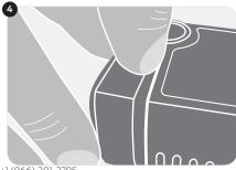
5. Remove the teardrop shaped stator by pulling up on the small lip.
